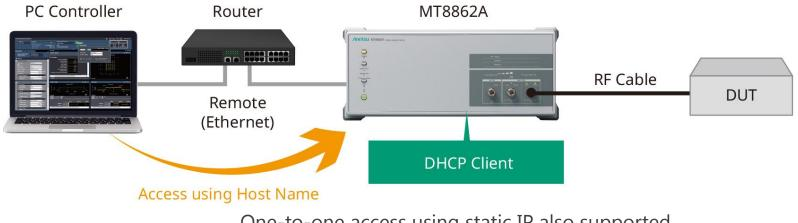
One-to-one access using static IP also supported
